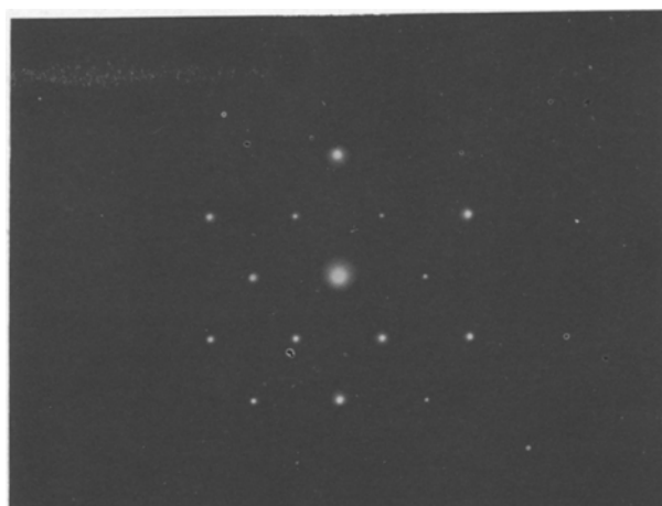
Figure 5 Selected area diffraction pattern of the same region as shown in Fig. 5.
